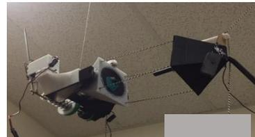
Figure 5; contents: *Spring separating system*
