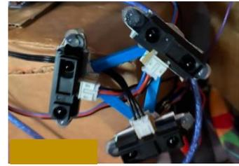
Figure 12; contents: *IR sensor triangle*
