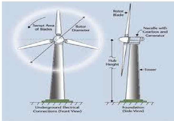
Drawing of the rotor and blades of a wind turbine, courtesy of ESH
