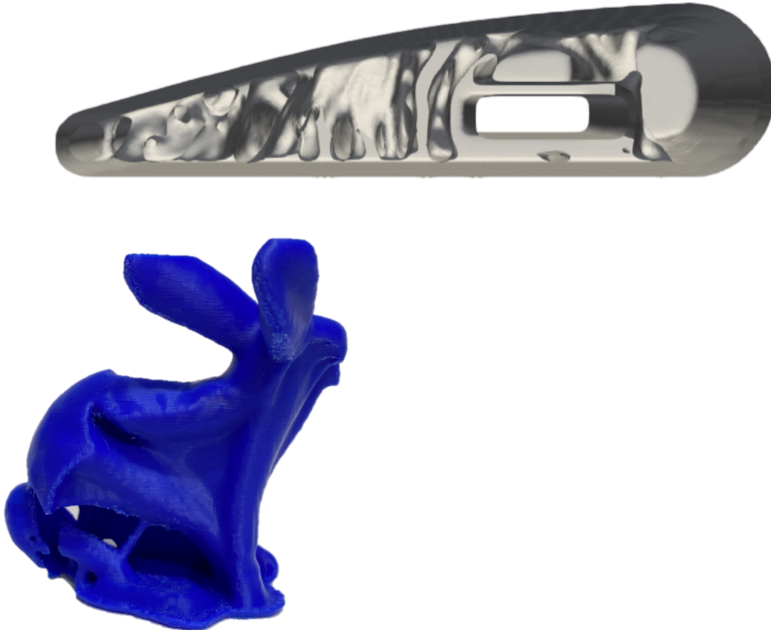
Figure 2: Topology-optimized parts by LANL, surface reconstructed using the software created for this project, and exported to 3D printers.
