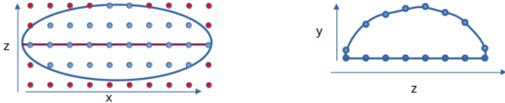
(a) Determining which points are within the bounds of the ellipse. (b) Finding y-coordinate for each point.
